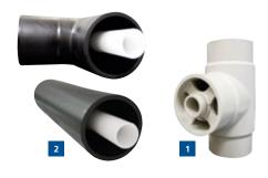
Factory fabricated double containment piping components are available in the standard supply range from: OD 90/32 mm - OD 355/250 mm. Special combinations are designed and produced project based.
